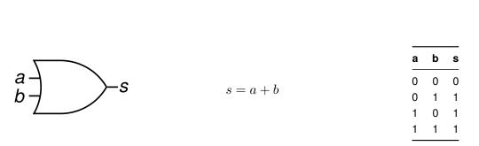
Note: x + 0 = x et x + 1 = 1, so an OR gate can be use to produce, from a signal x, a signal that equals to x or 1 depending on a command signal
